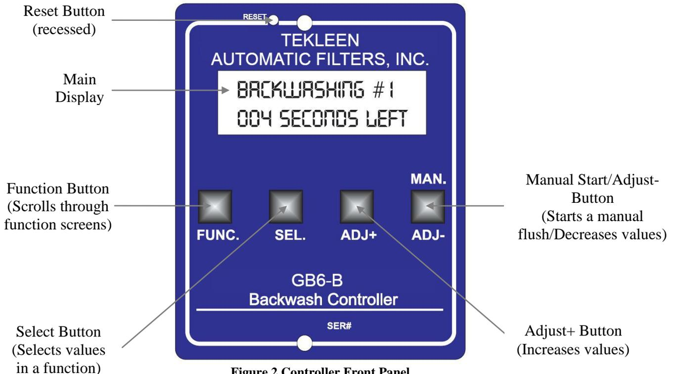
Figure 2 Controller Front Panel
